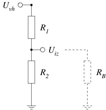
$$U_{iz} = \frac{R_2}{R_1 + R_2} U_{vh}$$
