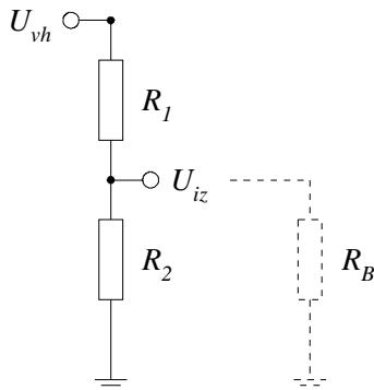
$$U_{iz} = \frac{R_2}{R_1 + R_2} U_{vh}$$
