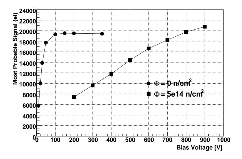
Most probable signal in [el] from Gain = 26.5 mV/fCDetector was annealed after irradiation for 80 minutes at 60 C. Measurements were taken at T  $\sim$  - 20C
