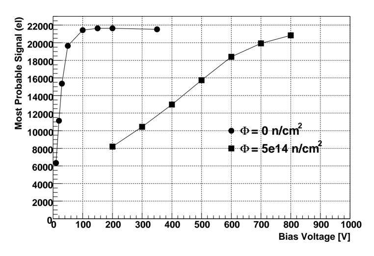
Detector was annealed after irradiation for 80 minutes at 60 C. Measurements were taken at T  $\sim$  - 20C
