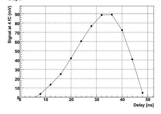
Pulse shape: signal vs. strobe delay for 4 fC calibration pulse
