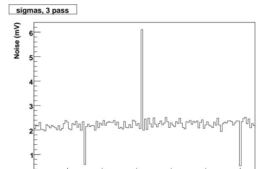
Noise vs. Channel number at the output of the test board (detector not yet connected. **Graph**
