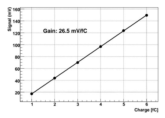
Response curve: average signal at the output of the test board from 32 channels vs. charge from on-chip calibration capacitors.
