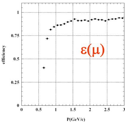
Fig. 109. Muon detection efficiency vs. momentum in KLM.
