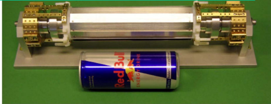
Prototype DEPFET pixel sensor and readout
