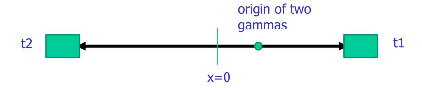
t1 = (L/2 - x)/c source at x, distance between detectors = L t2 = (L/2 + x)/ct1 - t2 = 2x/c
