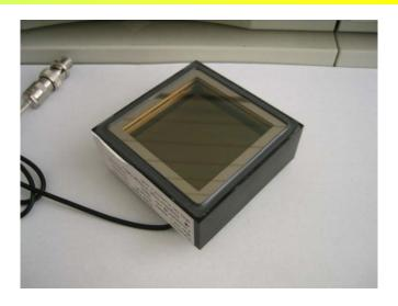
The main problem of a MCP PMT in a Cherenkov based annihilation gamma detector: low quantum efficiency of a typical photocathode in a PMT
