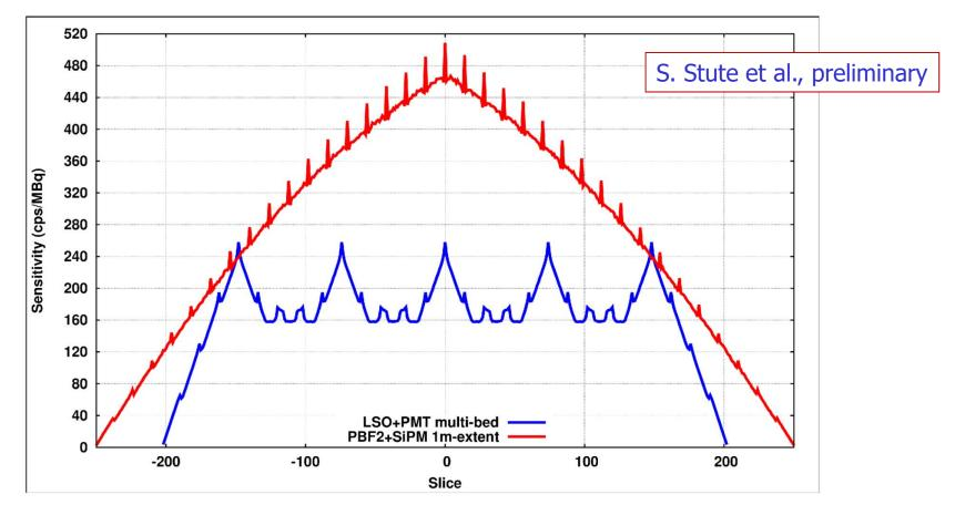
Axial sensitivity profiles following the NEMA standards at the center of the FOV, for the 1meter axial extent PbF<sub>2</sub>-based scanner and for a multi-bed LSO-based scanner.
