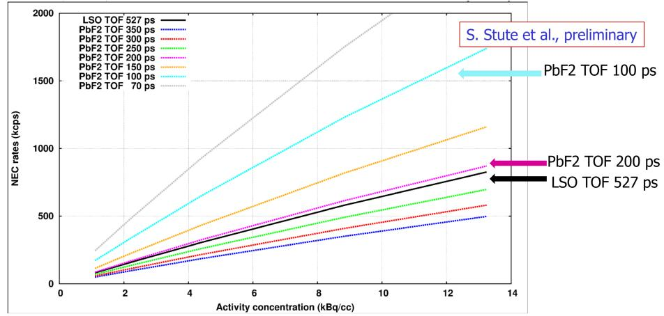
NEC rates for different activities and for the two scanners, following the Conti formula (with-TOF). Multiple TOF resolution are presented for the PbF<sub>2</sub>-based scanner.
