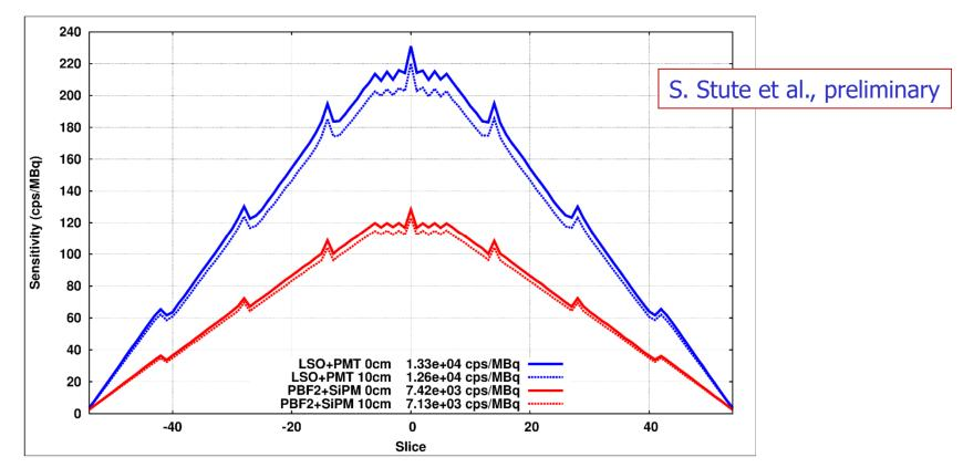
Axial sensitivity profiles following the NEMA standards, for the two scanners and at radial offsets of 0 and 10 cm; global sensitivity (all slices combined).
