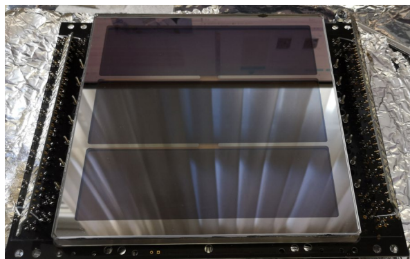
LAPPD with \text{PbF}_2 crystals
