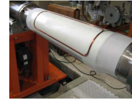
New superconducting / permanent final focusing quads near the IP
