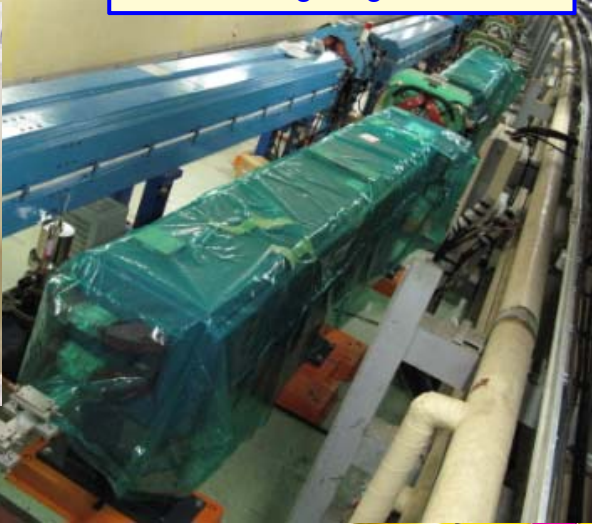
Installation of 100 new long LER bending magnets done
