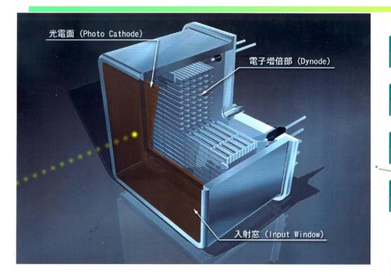
Multianode PMTs (MaPMTs) with metal foil dynodes and 2x2, 4x4 or 8x8 anodes Hamamatsu R5900 (and follow up types 7600, 8500)
