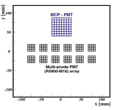
R5900-M16 characteristics: •bialkali photocathode •16 (4x4) pads, pitch 4.5mm •active area fraction ~ 36% •collection efficiency ~ 75%
