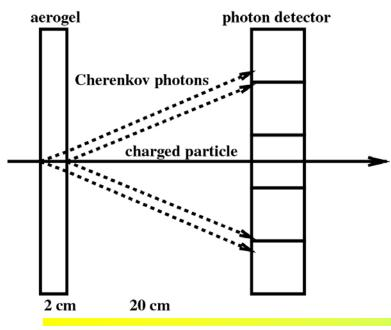
proximity focusing RICH with aerogel radiator in the forward direction
