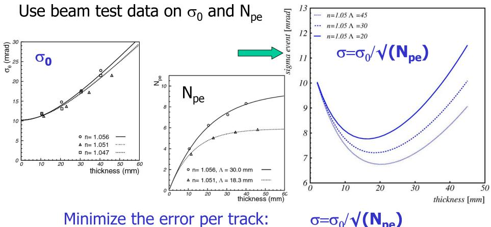
the error per track:  $\sigma = \sigma_0 / \sqrt{(N_{pe})}$ Optimum is close to 2 cm
