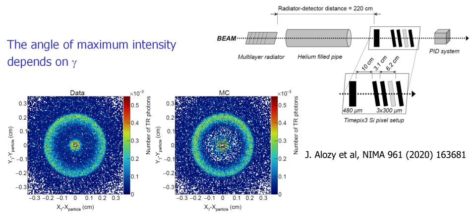
Figure 14: Relative position of identified TR photon clusters with respect to the particle clusters for  $20 \,\text{GeV/c}$  electrons crossing the polypropylene radiator. Left panel: data. Right panel: MC simulation.
