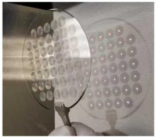
Compared to ordinary lenses: thin, lightweight, cheap, more flexible. Could be used to increase the active area of the detector (within limits given by the Louville's theorem).
