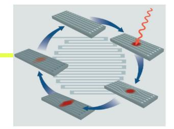
Example: superconducting nano-wire single photon detector (SNSPD): a thin (4 nm) and narrow (100-250 nm) superconducting nanostrip that is current-biased just below its critical current.
