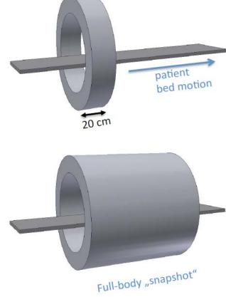
Simulations were performed in order to estimate the performance of TOF PET scanner based on the Cherenkov method of gamma detection.
