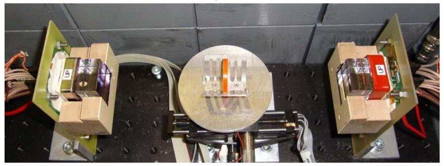
Cherenkov radiators: -monolithic: 25 x 25 x 5,15 mm<sup>3</sup> (PbF<sub>2</sub>, PbWO<sub>4</sub>) -4x4 segmented: 22.5x22.5x7.5 mm<sup>3</sup> (PbF<sub>2</sub>) -black painted, Teflon wrapped, bare
