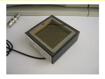
The main problem of a MCP PMT in a Cherenkov based annihilation gamma detector: low quantum efficiency of a typical photocathode in a PMT
