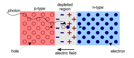
Photo-diode: (visual) photon is absorbed in the depleted region, produces an electron-hole pair.
