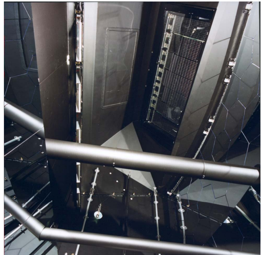
System of mirrors of the HERA-B RICH
